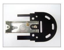
The base end cap plate is first held in position on to the architrival back box through either of the slots in the plate. One slot allows longitudinal movement the other horizontal if fitting to paired box ends. As above, once the end cap plate is held in position on the architrave box the wall can be marked for drilling. Remove plate to enable drilling and plugging. Proceed with the wiring and cover plate fitting as in No1
